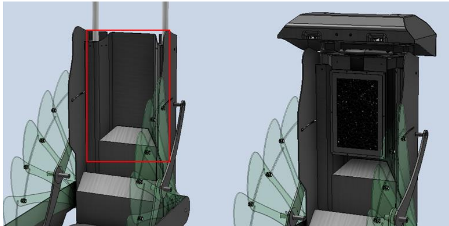
Figure 22: Recessed space in the body allocated for the screen when in the retracted position
