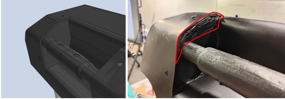
Figure 27: A 20mm gap introduced after bending acrylic had to be filled in. (Left: Computer model, Right: Physical prototype)
