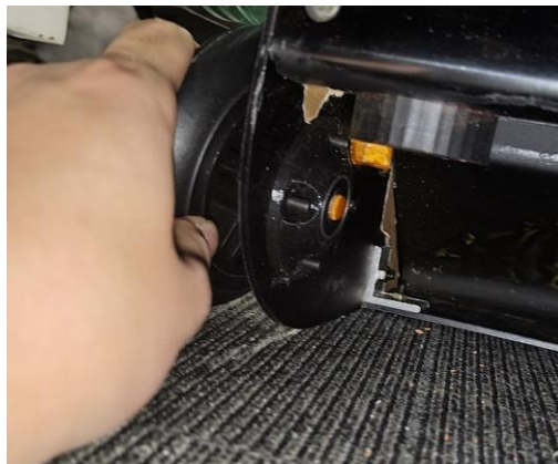
Figure 28: Bending of the 3D-printed bearing holder (black) when a torque is applied to the wheel perpendicular to its axis.
