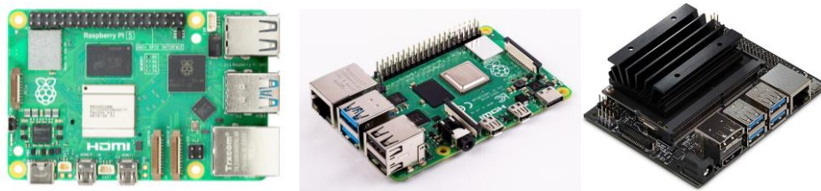
Figure 24: 3 Models of microcontroller boards: (Left: Raspberry Pi 5, Middle: Raspberry Pi 4, Right: Jetson Nano)
